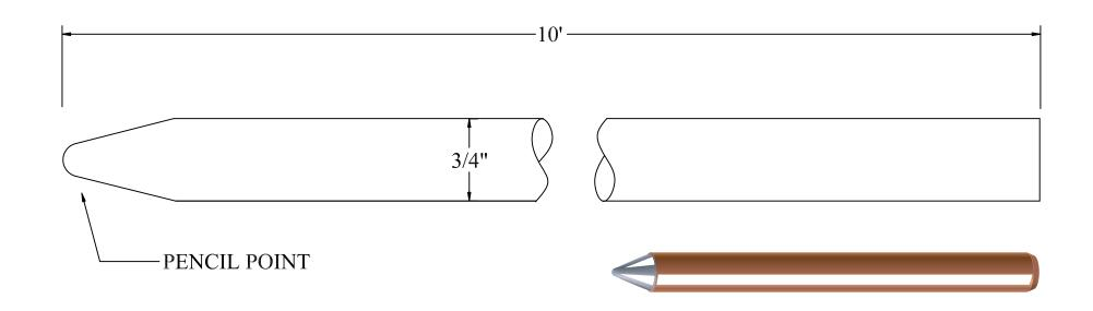
**Copper Clad Ground Rod**
