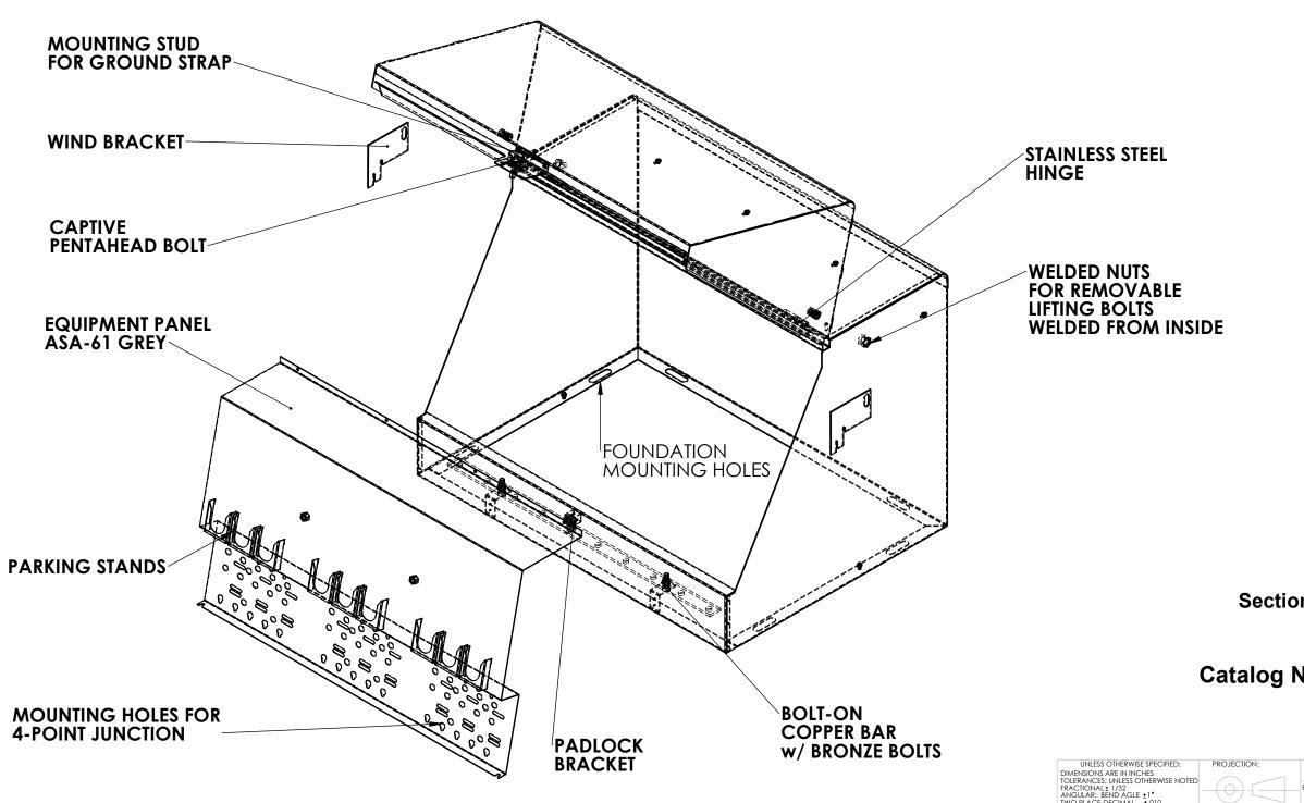
Sectionalizing Enclosure, 3-Phase, 28kV (30"H x 42"W x 30"D)
